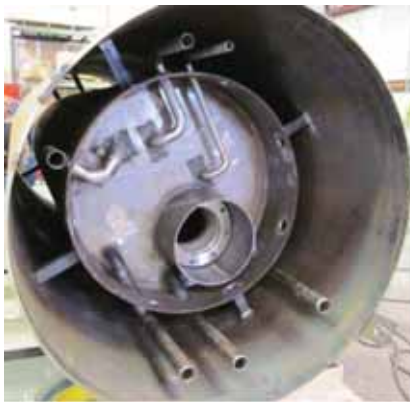
The end view of the Shielded Ion Exchange Module (SIXM) with the shielding annulus shown in Avantech's manufacturing facility.
